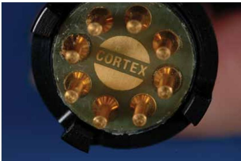
**Figure 2.** The corneometry probe consists of several pins used to measure the ability of skin to conduct electricity, an indirect measurement of cutaneous hydration.
