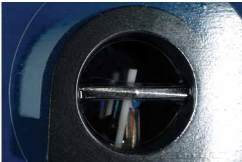
**Figure 1.** This close-up view of the transepidermal water loss probe shows the humidity meters in the chamber through which the water vapor must flow to obtain an accurate measurement.
