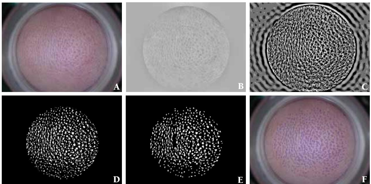
**Figure 3.** Image analysis software for analyzing pores, depicting source color image (A), gray level image (B), high-frequency image (C), binarised image after morphologic operations (D), image after final geometric filtering (E), and color image with detected pores (F).
