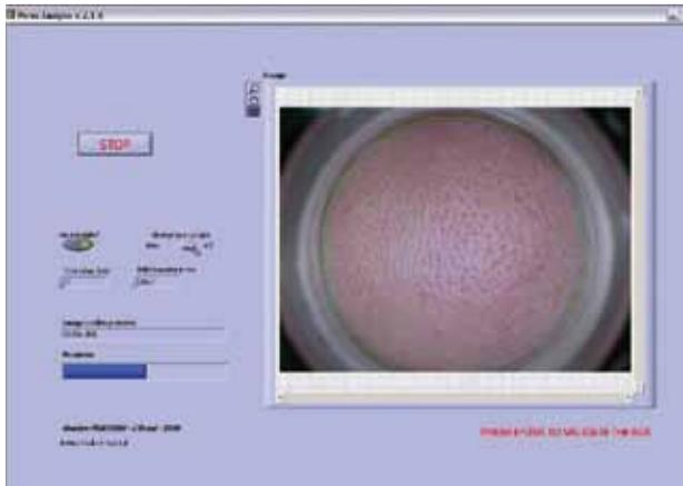
**Figure 2.** User interface of image analysis software for analyzing pore size.
