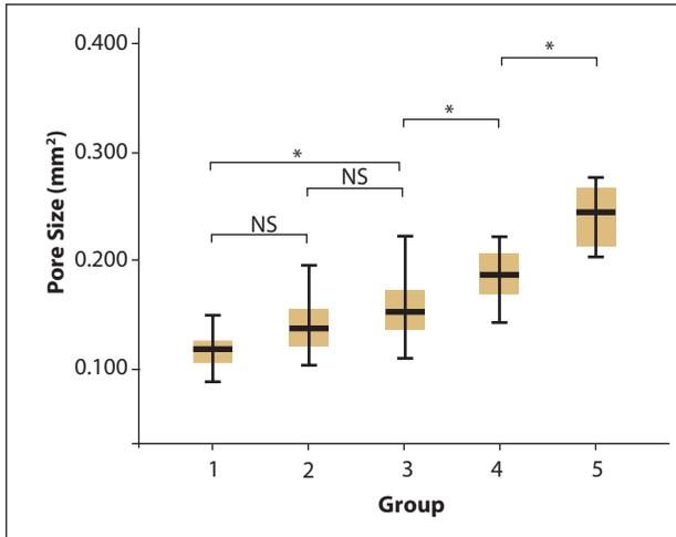
**Figure 5.** Mean pore size (mm<sup>2</sup>) measured by image analysis software for each group, with a 250- $\mu$ m threshold. Asterisk indicates significant differences at  $P < .05$  level; NS, no statistical differences between groups.
