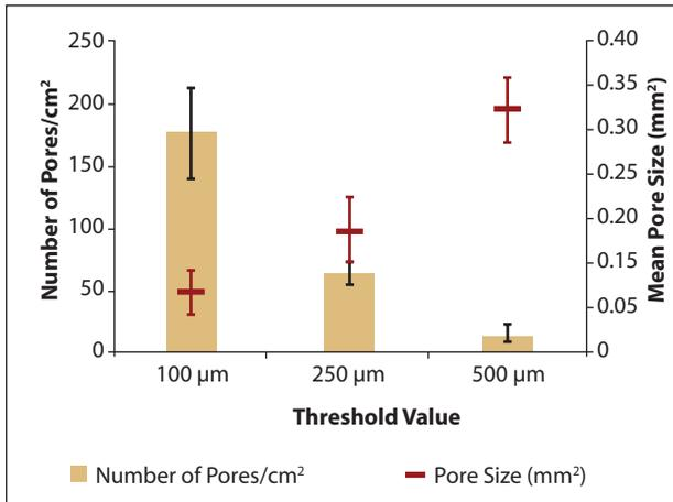
**Figure 6.** Size and number of detected pores (mean calculated on all the images) versus threshold value.
