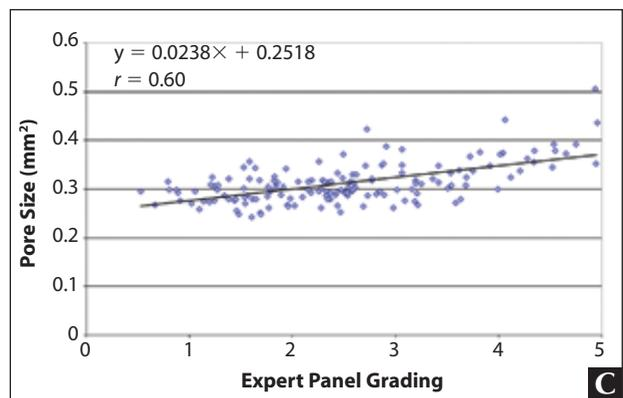
**Figure 4.** Pore size measured by image analysis versus expert panel grading, with thresholds of 100 µm (A), 250 µm (B), and 500 µm (C).
